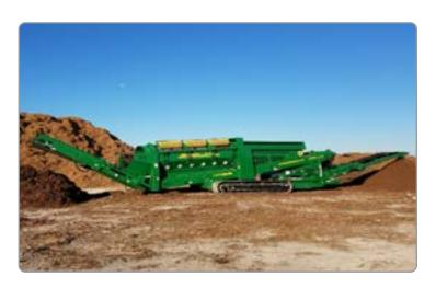
OVERSIZE CONVEYOR Heavy duty oversize conveyor at the end of the trommel offers adjustable speed and stockpile height.
