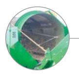
BRUSHES Ground level adjustable brushes keep the screen clean and rotate away from drum for ease of drum change.
