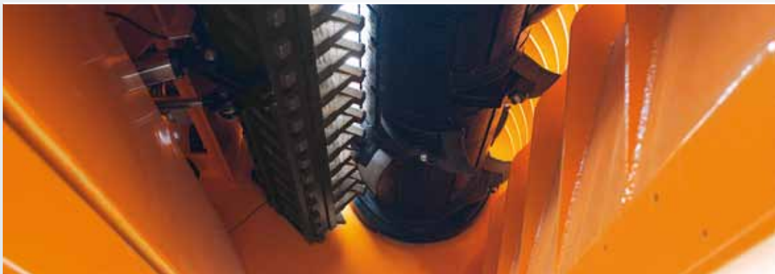
Shredding roller with hydraulically controlled shredding comb
