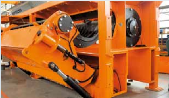
Hydraulically opening comb of the DW 306
