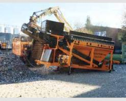
The ball coupling enables the machine to be moved on site easily, e. g. by a wheel loader grab. By means of the adjustable supports the height can quickly be adjusted to different shredder for direct feeding.
