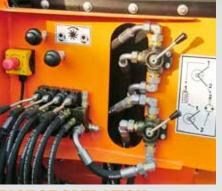
The machine is controlled from one central point ensuring ease of operation. No electric system, just hydraulic and manual control of all the required functions.
