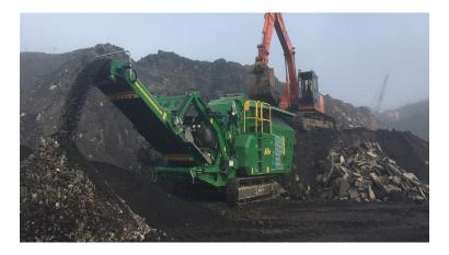
CONVEYORS Integrated hydraulic folding stockpiling conveyors.
