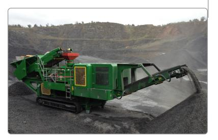
ADJUSTABLE FEEDER CONVEYOR Control panel, remote, or fully automatic regulation allows optimal operation of the crusher to better control the product material.
