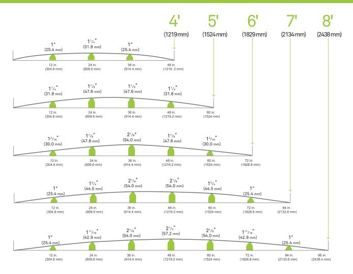
For other widths, the optimal curve for a crowned deck can be calculated by our inside sales personnel. Only with proper assessment the correct adapters for the crowned deck modifications can be ordered and installed.
