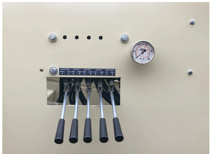
10/ HYDRAULIC CONTROL CENTER
