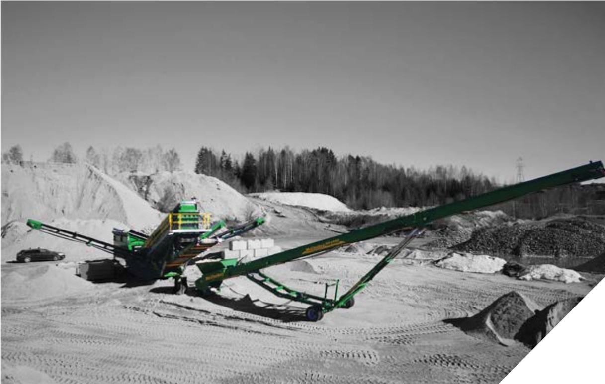
The WS4065 is a wheeled stacker that was designed to allow operators to stockpile/transfer material and complements our existing range of mobile crushing and screening plants. It offers a low-cost solution to stockpiling material, where space is at a premium.
