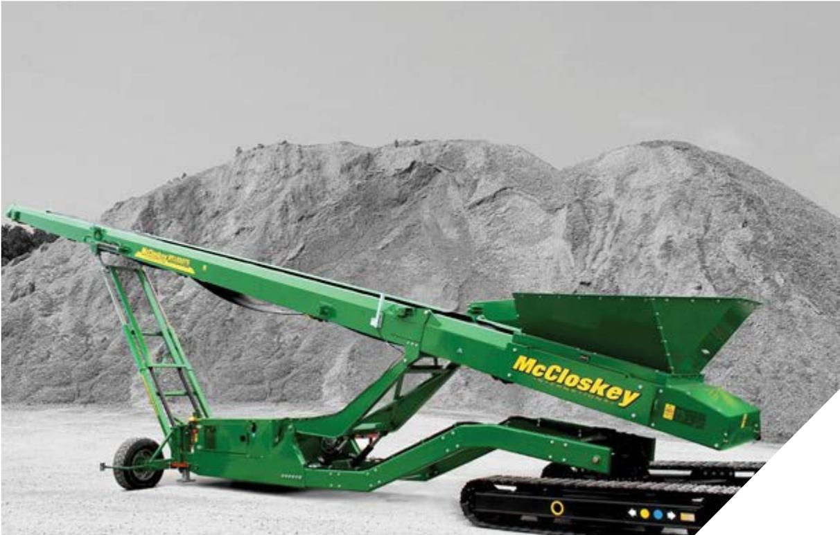
The WS4080TR combines the mobility of the WS4080 with the additional stockpiling options a radial tracked machine provides.
