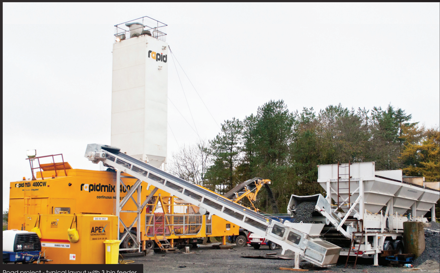
Road project - typical layout with 3 bin feeder
