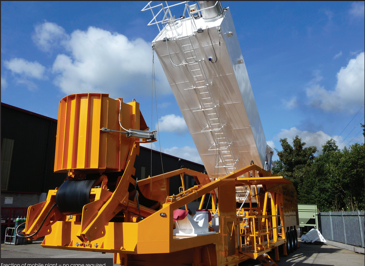
Erection of mobile plant – no crane required
