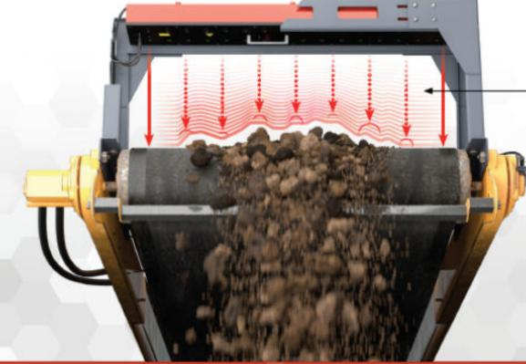
Secondly, the sensor measures the feed rate of the conveyor belt by an inductive sensor. Finally, by combining the cross profile and feed rate measurements, the resulting material data is readily available in cubic meters, yards or tonnes, and stored in the Sensor for easy download.
