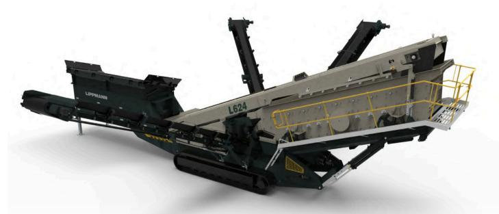
The heavy duty tracked mounted mobile screener offers options of single or double deck live head, single shaft shredder, 12' or 15' hopper, and crusher feed in chute (only in conjunction with 15' hopper). The safety feature list includes external belt alignment points, external grease points, engine safety shutdown systems, and full safety guarding for nip points.
