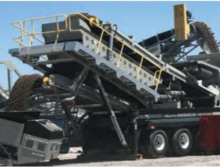
Hydraulically adjustable screen angle allows you to select the appropriate angle for your application. The spreader split ensure material is evenly deposited on the vibrating screen.
