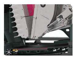
The large gap between crusher discharge and main conveyor belt, paired with wide main and side conveyors result in an optimized material flow.
