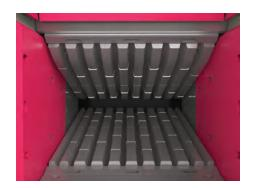
Deep 75" (1.91m) jaw chamber with single toggle design accommodates hard rock applications and large feed sizes. Also features closed side setting adjustment with hydraulic wedges.
